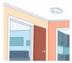
The smoke alarm should be attached to the ceiling.
