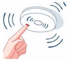
Test the smoke alarm every month by pressing the test button.
